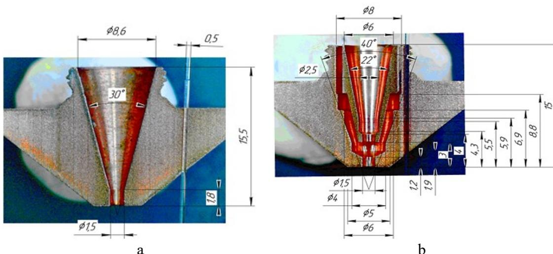
**Figure 4.** Configuration and geometric dimensions of Thermacut's standard single-channel (a) and dual-channel (b) nozzles with a center bore diameter of 1.5 mm
